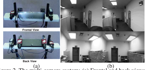
Figure 2. The multi-camera system: (a) Frontal and back views of the system; (b) Captured images of both stereo pairs.
