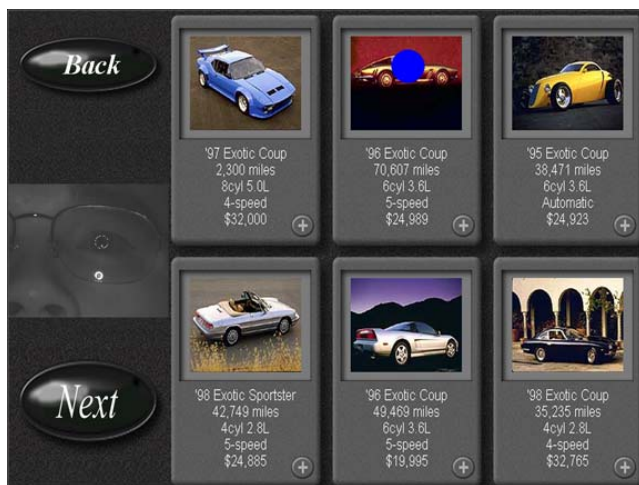
Fig. 16. Cars for the selected car option in Fig. 15. Another selection is made by gazing on this image as indicated by the shaded circle to indicate the specific car that the user has an interest in. The user can view other “exotic” cars’ information by looking at the “Next” button or browse other types of cars by looking at the “Back” button
